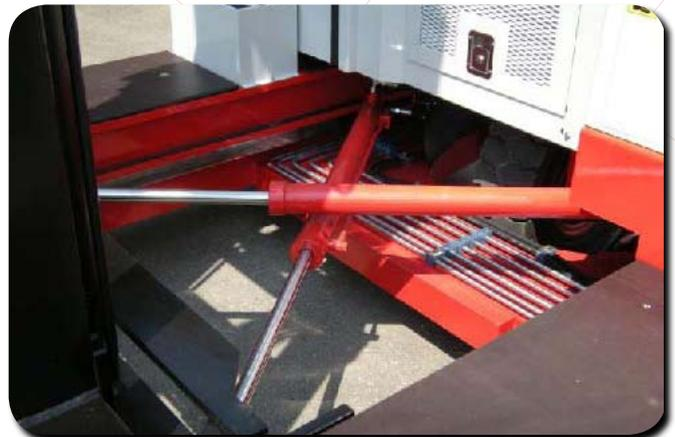
BP utilizes a cross system of hydraulic pistons for smooth even positive control of the mast.
