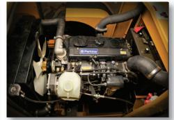
**ENGINE:** The P Series forklifts have a sliding hood for easy access during maintenace, and house a Perkins Turbo Tier 3 emissions compliant diesel engine.
